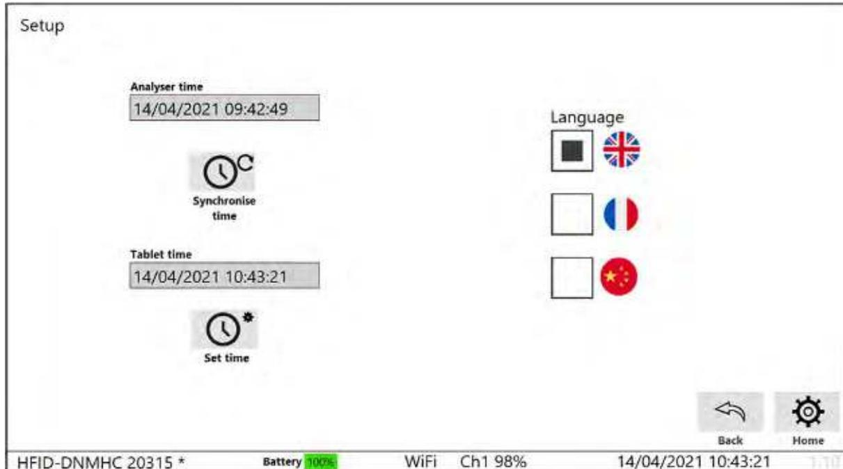
**Figure 19 : Tablet GUI - Time/language setup screen**
