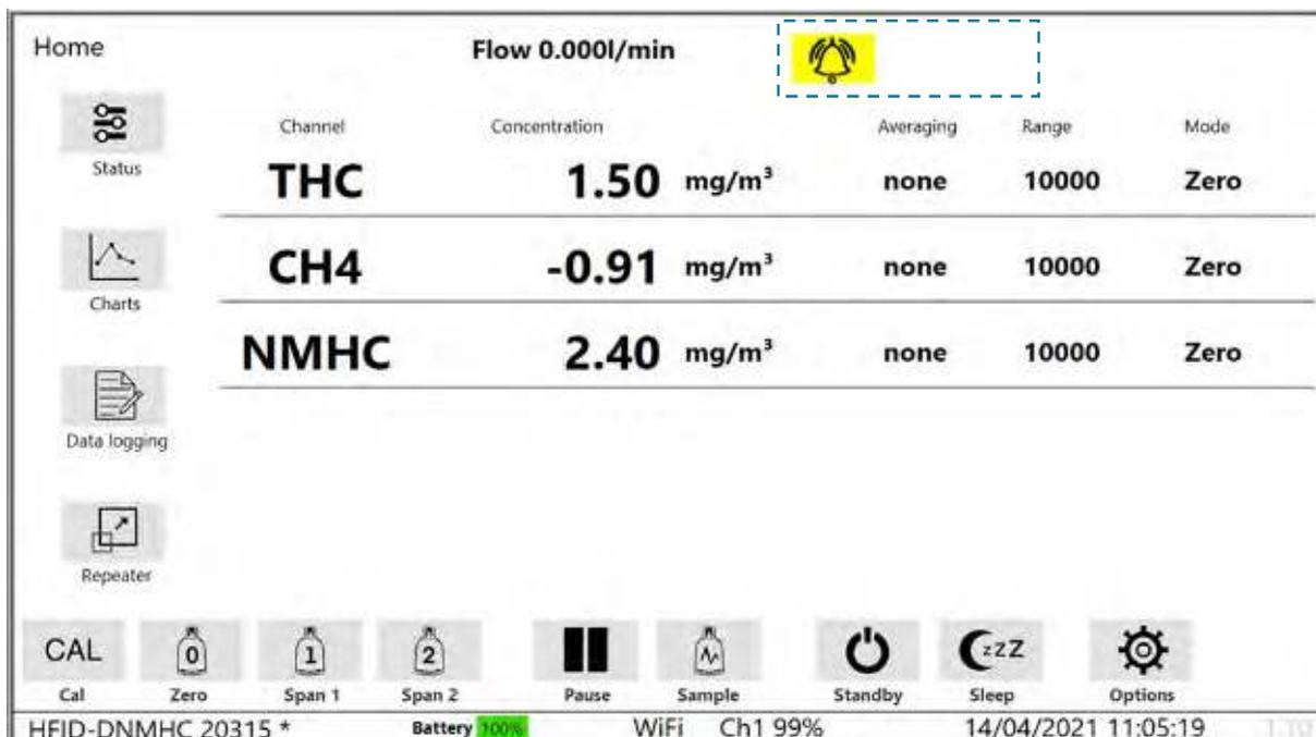
Figure 18 : Tablet GUI - Home screen with Alarm
