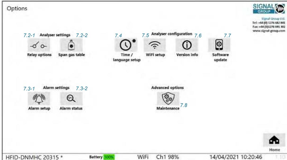
Figure 13 : Tablet GUI - Options screen
