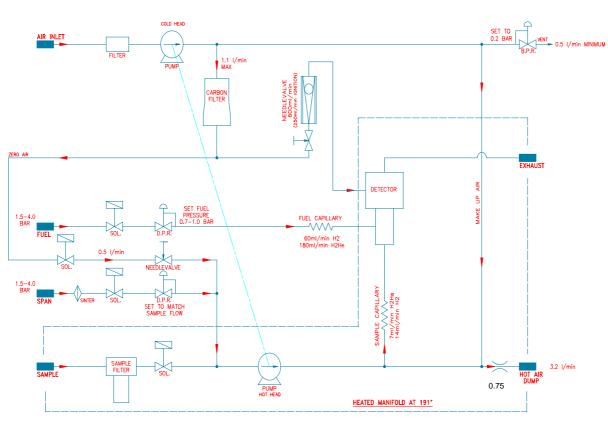
NOTES:-1) COLD HEAD SHOULD PROVIDE NOT LESS THAN 4.5 I/min. INTO 0.2 bar. 2) ALL READINGS STATED ARE NOMINAL FIGURES.
