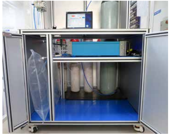
THC measurement setup at MAHLE
