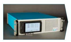
Rack mounted FID for continuous monitoring
