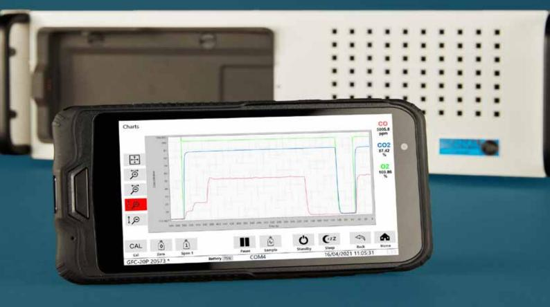
Detachable wireless tablet is compatible with S4 gas analysers suitable for local and remote operation.
