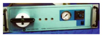
This compact 3U high 19"rack enclosure houses the 340 Distribution oven including a particulate filter and needle-valve manifold arrangement filter.
