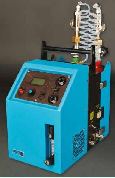
Portable Flame Ionisation Detector (FID) analysers for the discontinuous measurement of the mass concentration of gaseous and vaporous organic substances in stationary source emissions.
